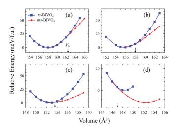
FIG. 3. (Color online) Relative energies per formula unit (f.u.) for ts-BiVO<sub>4</sub> and ms-BiVO<sub>4</sub> with respect to the lowest energy structure of ts-BiVO<sub>4</sub> as a function of volume calculated using (a) pure PBE, (b) PBE-HF10%, (c) PBE-HF25%, and (d) PBE-HF50%. For each case, the crossover volume ( $V_C$ ) where the energy-volume curves of ts-BiVO<sub>4</sub> and ms-BiVO<sub>4</sub> meet is indicated by the arrow.
