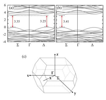
FIG. 7. (Color online) Band structure diagrams for (a) ts-BiVO<sub>4</sub> and (b) ms-BiVO<sub>4</sub> from PBE-HF25% calculations, together with (c) Brillouin zone for a body-centered tetragonal crystal structure. The bands are plotted along  $\Sigma$  and  $\Delta$  directions as specified in (c); for each case, the energy zero is set at the top of the valence band. The direct/indirect band-gap values are also indicated.
