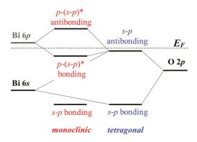
FIG. 2. (Color online) Schematic representation of the interactions between Bi 6s, Bi 6p, and O 2p orbitals in ts-BiVO<sub>4</sub> (in blue) and ms-BiVO<sub>4</sub> (in red). The asterisk (\*) denotes an antibonding state, and the dashed horizontal line indicates the Fermi level ( $E_F$ ).
